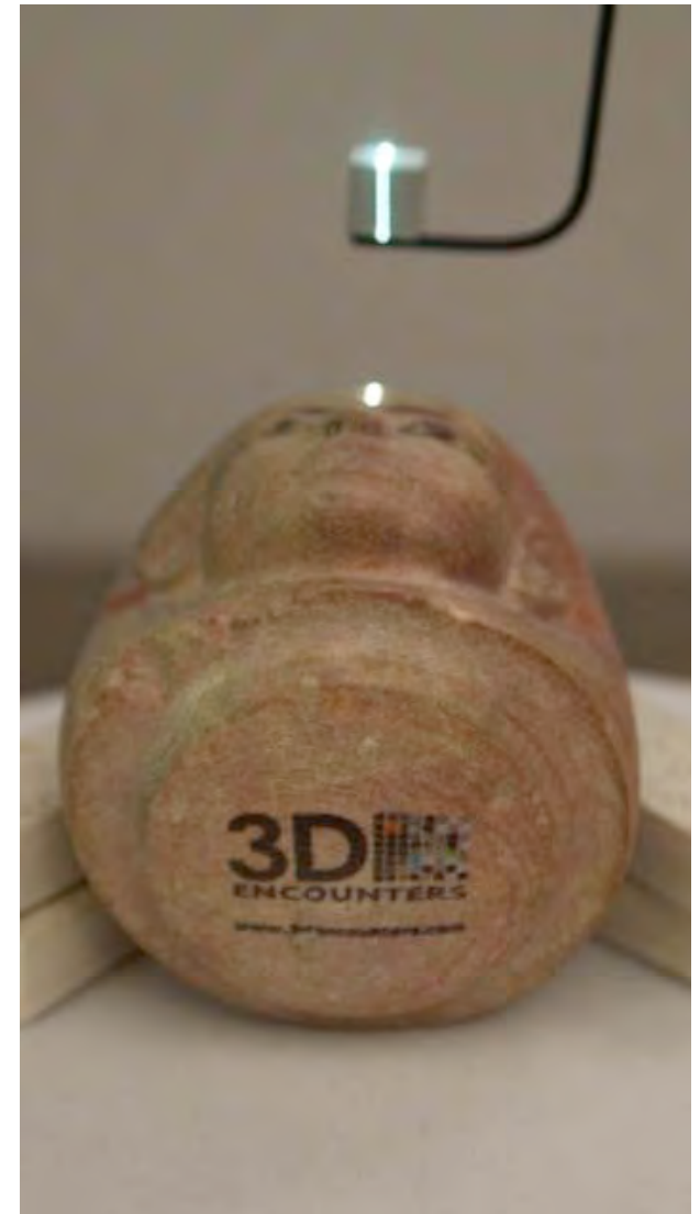
An object being scanned: the white cube controls light and colour
